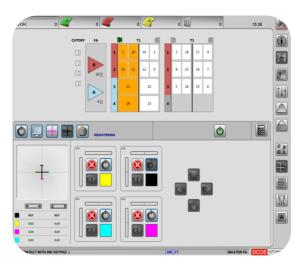
Support for a wide range of optional modules can extend the user interface even further to integrate with auxiliary equipment, such as splicers, remote ink, dampening and closed-loop systems. This will make the printing machine as a whole easy to operate through the same software with the same look and feel.
